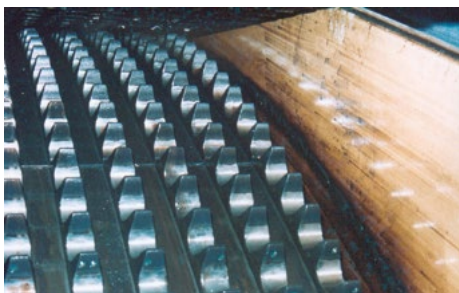
Ruota a 6 corone, 3" e 197 denti 3" and 197 teeth sixfold wheel Rueda de 6 aros, 3" y 197 dientes
