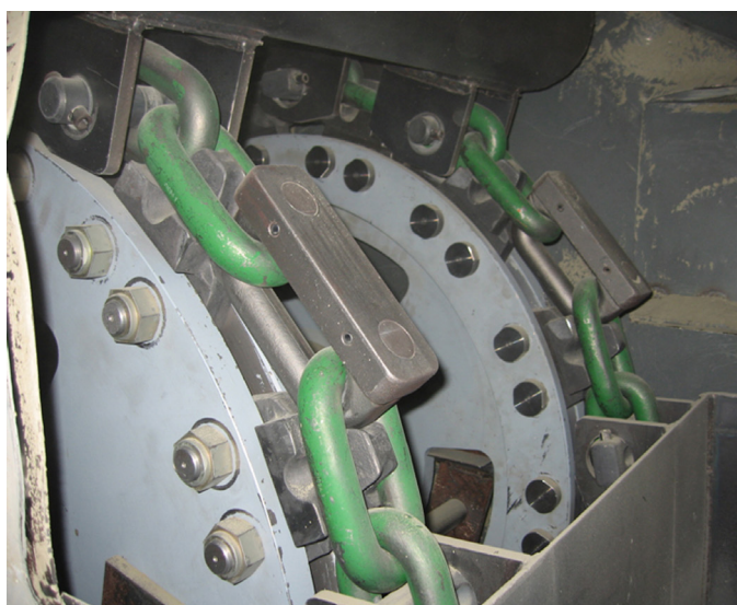
Figure 5. Driving station of a toothed wheel bucket elevator with Ø34 mm CICSA LH-CS chain and GV34 couplings.
