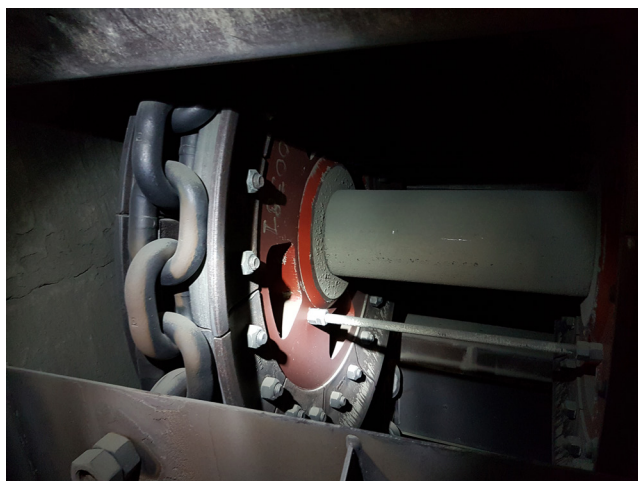
Figure 2. An example of a CICSA smooth drive wheel with replaceable forged segments (RLS type).
